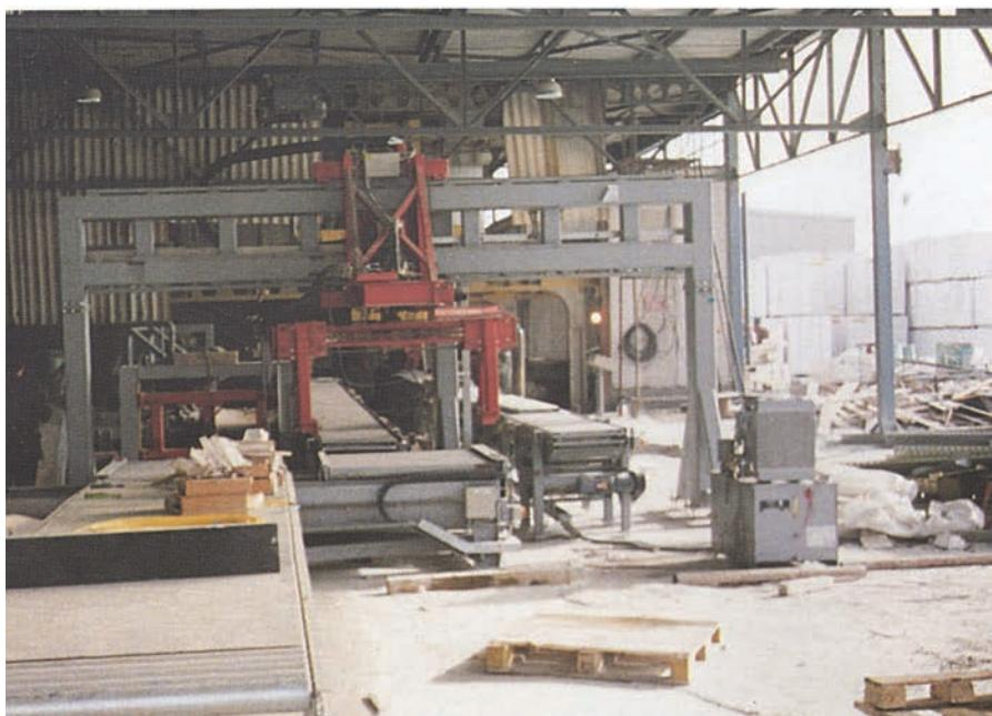
The electrical and mechanical installation and start up of 75 tons of machines and equipment under the supervision of Dutch Aarding firm for a factory producing gasconcrete elements in İstanbul, within 20 days.
